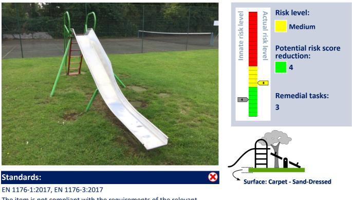
The item is not compliant with the requirements of the relevant standards. The surfacing meets with the requirements of the relevant standards.
